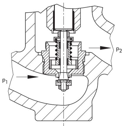
Type 2405 **without** pressure balancing ( $K_{VS}$  0.016 to 1)
