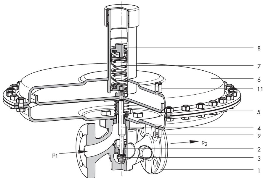
Type 2405 **without** pressure balancing ( $K_{VS}$  1.6 to 4) · Flow-to-open
