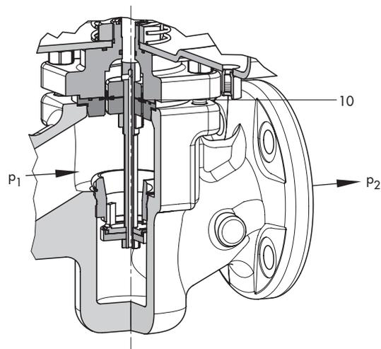
Type 2405 **with** pressure balancing ( $K_{VS}$  6.3 to 32)
